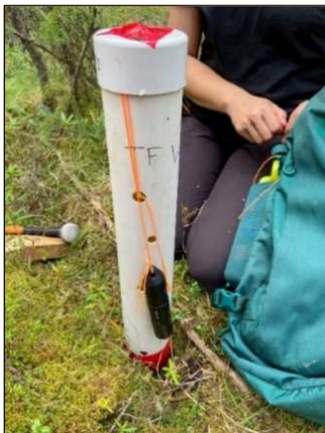
Figure 14. Barometric data logger (bottom center) attached to the outside of a well.
